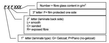
Example: GCF600 = Gelcoat laminate protected by Film and with back side sanded surface. Produced with 600 g/m² of fiberglass.
